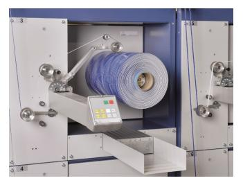
With its unmatched versatility, the **SAHM 460XE Series** can accommodate a wide variety of bobbin types – including cylindrical, cops, diabolo, pancake, step winding, delta stepwinding, flange tubes, and cross-winding configurations. This adaptability makes the 460XE Series ideal for diverse applications such as foamed tapes for sealing and insulation, towpreg and prepreg tapes used in composite manufacturing, and pitch-based carbon fiber designed for high-tech applications.
